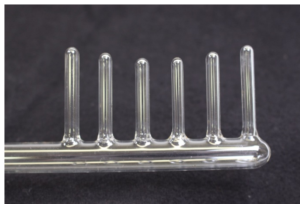
Fig. 6: The comb electrode named by the donor (detail)
