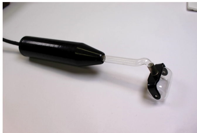
Fig. 10: Velmag Frequenta – handle with attached roller electrode
